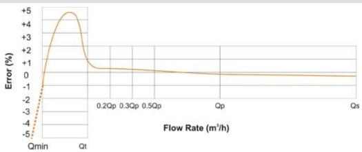
Error in the low flow zone from Qmin to Qt is  $\pm 5\%$ . Error in the upper zone from Qt to Qs is  $\pm 2\%$ .
